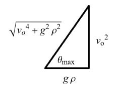
Finally, plug  $\theta_{\text{max}}$  into the formula for the projectile's height to get the equation of the surface that marks the furthest the projectile can reach.
